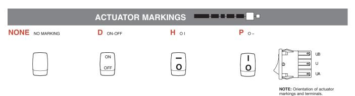
'D & P' marking options: marking color white, standard for all actuator colors except white actuators. Black marking color standard for white actuators. Consult Customer Service Center for other available marking colors.
